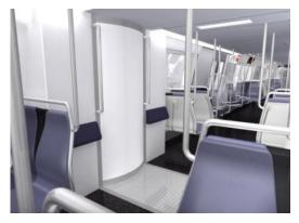
the cars could be used to create an open gangway within the married pair. These should be flexible/moveable to allow the cars to shift and turn apart from each other, yet durable enough to withstand a rail environment and passenger wear and tear.
